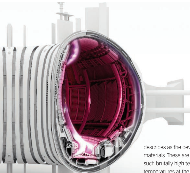
Computer cut away of JET: finding suitable materials for the glowing divertor at the bottom of the ring, as well as the inner walls, continues to challenge
